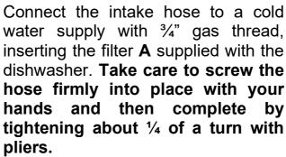
In dishwashers equipped with the AQUASTOP device, the filters is already fitted inside the threaded ring.
