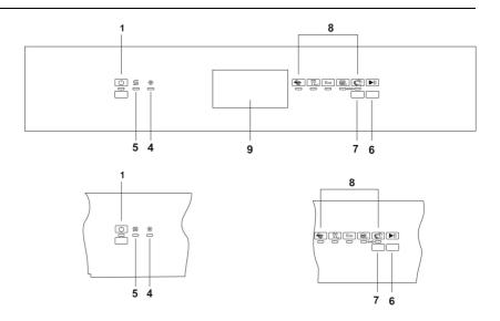
**ON/OFF** BUTTON AND WARNING LIGHT 2 Not present 3 Not present **SALT WARNIN LIGHT** 4 **NO RINSE AID LIGHT** 6 **PROGRAM SELECTION BUTTONS** START/PAUSE BUTTON 7 8 **PROGRAM INDICATOR LIGHTS** HANDLE TO OPEN THE DOOR 9
