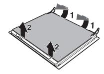
3. Some models are fitted with a pair of intermediate glass panes. Remove the intermediate glass panes by lifting them upwards.
