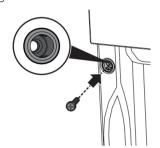
4. Cover the bushings with the previously removed covers.
