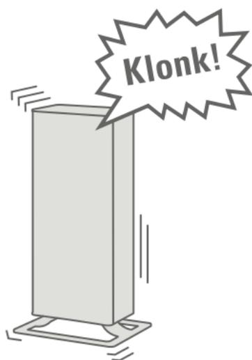
**EN** Important advice: If you hear a «klonk» noise from the appliance, it is the tip-over-switch which stops the heater in case it topples over.
